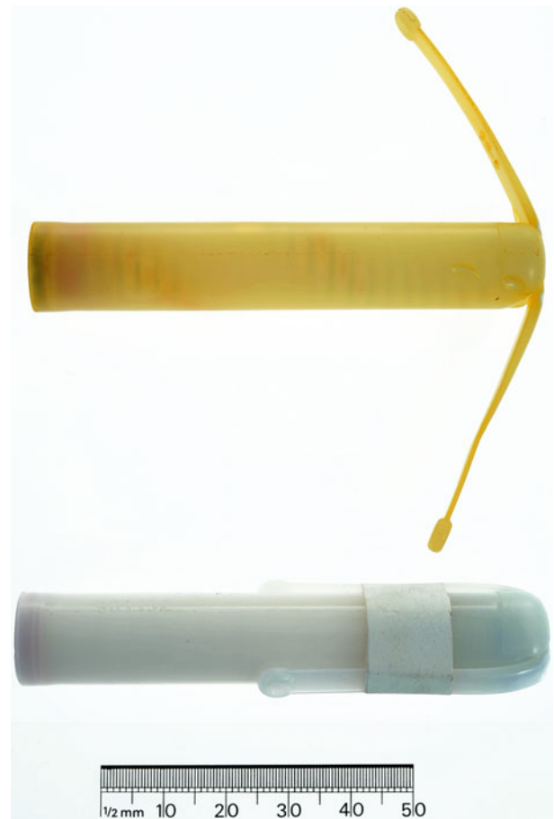
Fig. 3. Photo of the delayed-release intra-ruminal bolus before administration (bottom) and after recovery from the rumen following successful release of all anthelmintic tablets (top).
