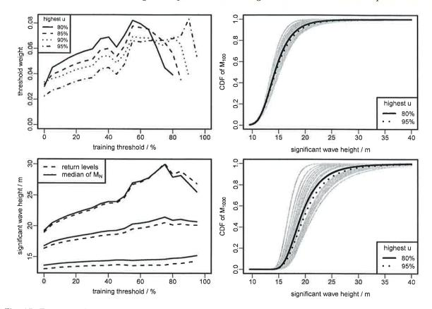
**Fig. 15.** Extreme value inferences for the Gulf of Mexico data using a Cauchy prior for  $\xi$ . Top left: estimated threshold weights by the highest training threshold. Bottom left: *N*-year predictive return levels and medians of the predictive distribution of  $M_N$  for N = 100,1000 and 10000. Right: threshold-specific (grey lines) and threshold-averaged (black lines) predictive distribution functions of  $M_{100}$  (top) and  $M_{1000}$  (bottom).
