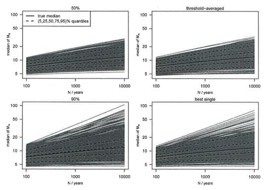
**Fig. 9.** Exponential example. Predictive median of  $M_N$  by N: individual datasets (grey), N-specific (5,25,50,75,95)% sample quantiles (dashed) and true median (solid). Threshold strategies: median (top left); 90% quantile (bottom left); threshold-averaged (top right); 'best' threshold (bottom right).
