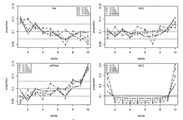
**Fig. 4.** Proportions of simulated values of  $\widehat{P}(M_N \leq z_{\text{new}} \mid x)$  falling in U(0,1) deciles for the case  $\xi = 0.1$  and  $p_u = 0.5$ . The prior is labelled on the plots. Separate lines are drawn for N = 100, 1000, 10000 and 100000. 95% tolerance limits are superimposed.
