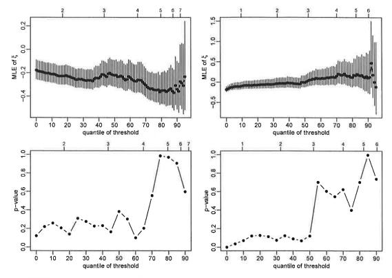
**Fig. 2.** Threshold diagnostic plots for the storm peak significant wave height hindcast datasets. Left: North Sea data. Right: Gulf of Mexico data. Top: parameter stability plots for MLEs of  $\xi$ , with 95% pointwise profile likelihood-based confidence intervals. Bottom: *p*-values associated with a test of constant shape parameter against the lowest threshold considered. The upper axis scales give the level of the threshold in metres.
