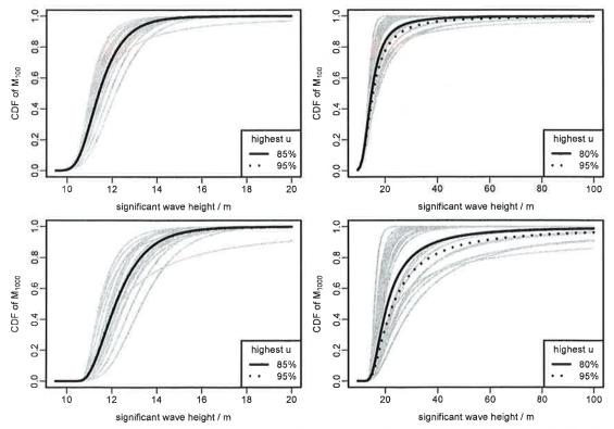
**Fig. 13.** Threshold-specific (grey lines) and threshold-averaged (black lines) predictive distribution functions of  $M_{100}$  (top) and  $M_{1000}$  (bottom). Left: North Sea data. Right: Gulf of Mexico data.
