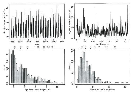
**Fig. 1.** Storm peak significant wave height hindcast datasets. Left: North Sea data (628 observations). Right: Gulf of Mexico data (315 observations). Top: time series plots. Bottom: histograms. The upper axis scales give the sample quantiles.
