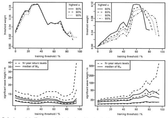
**Fig. 7.** Analyses of significant wave height data by training threshold *u*. Top row: estimated threshold weights by the highest training threshold considered. Bottom row: *N*-year predictive return levels and medians of the predictive distribution of  $M_N$  for N = 100, 1000 and 10000. Left: North Sea. Right: Gulf of Mexico.
