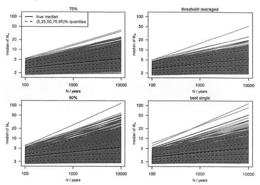
Fig. 11. Uniform-GP hybrid example. Predictive median of M<sub>N</sub> by N: individual datasets (grey), N-specific (5,25,50,75,95)% sample quantiles (dashed) and true median (solid). Threshold strategies: 75% quantile (top left); 90% quantile (bottom left); threshold-averaged (top right); 'best' threshold (bottom right).
