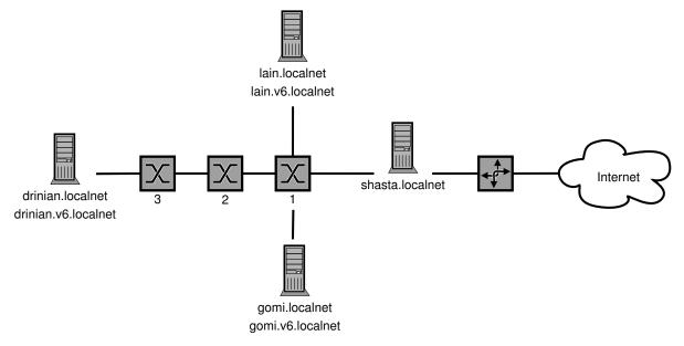
Figure 6.1: Test network layout.
