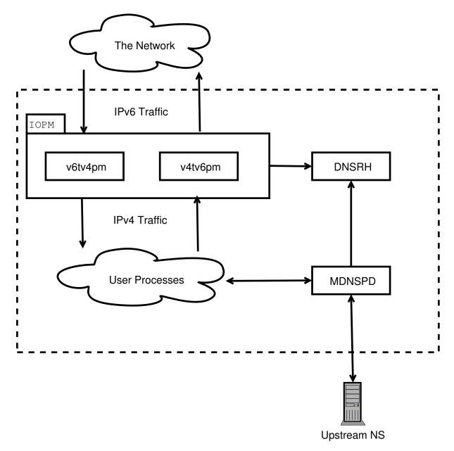
Figure 4.2: Non-Implementation specific detailed architecture diagram.
