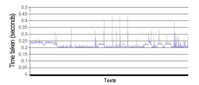
Figure 6.4: Proxying v4 requests via the test machine, over 2000 hosts.
