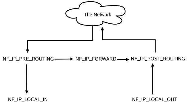
Figure 3.1: Structure of netfilter hooks [47].
