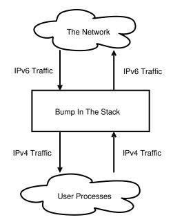
Figure 4.1: A simple overview of the BIS architecture
